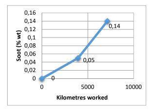
**Graph 3** Soot content in the engine oil depending on the mileage of the oil level Source: authors.
