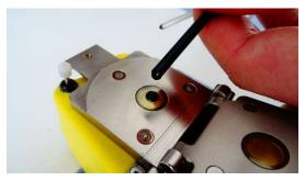
**Fig. 8** Inserting the sample on the sample slide 1 Source: authors.
