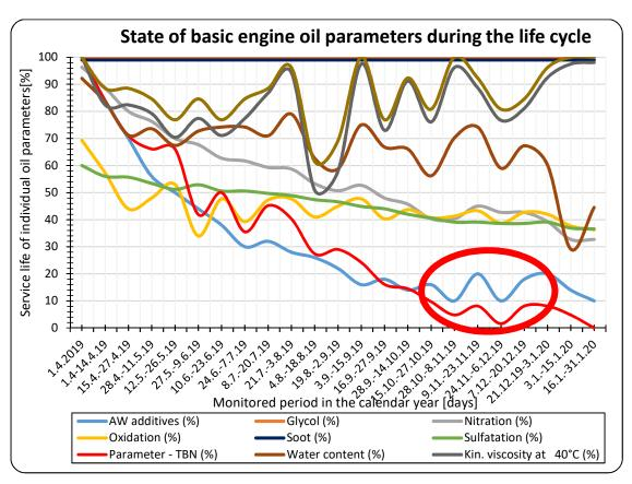
Fig. 5 Illustrative example service life of engine oil in an internal combustion engine and the most fragile parameters (parameter TBN, AW additives) [1]
