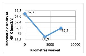
**Graph 5** Change in kinematic viscosity of the engine oil at 40 ° C depending on the kilometers of oil filled Source: authors.
