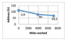
**Graph 1** The level of motor oil addition depending on the mileage of the oil level Source: authors.
