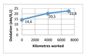
Graph 2 The level of oxidation of the engine oil depending on the kilometers of oil filled Source: authors.
