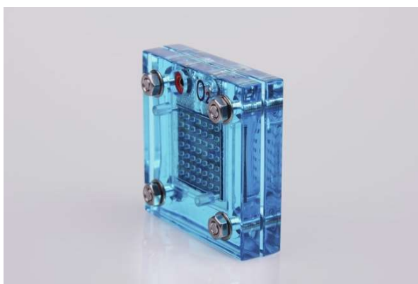
Fig. 2 Example of fuel cell using Nafion membrane Source: [4].
