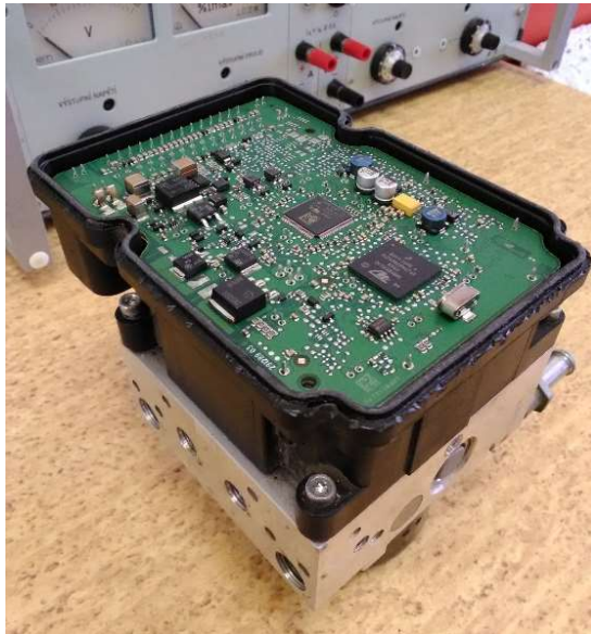
Fig. 3 Disassembled faulty hydraulic unit with integrated regulator (hydraulic control modulator) Source: authors.
