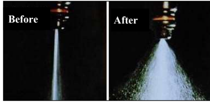
Fig. 2 Injector operation before and after the use of additive (illustrative photograph) Source: [7].
