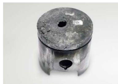
Fig. 1 Damaged piston (illustrative photograph) Source: [11].
