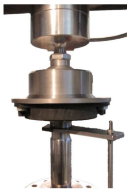
Fig. 1 Damper mounting on test rig
