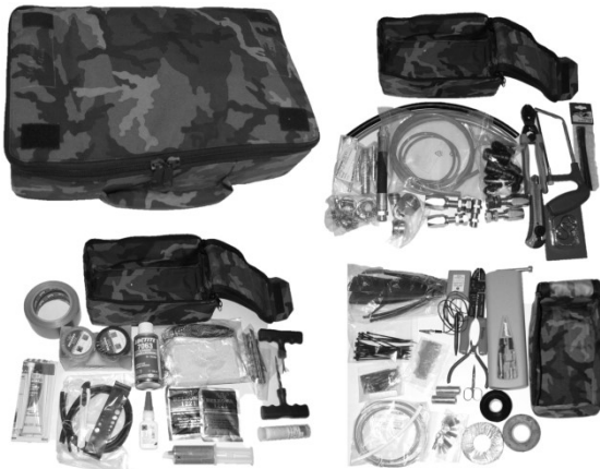
Fig. 3 Battle damage repair kit for repair land combat vehicles
